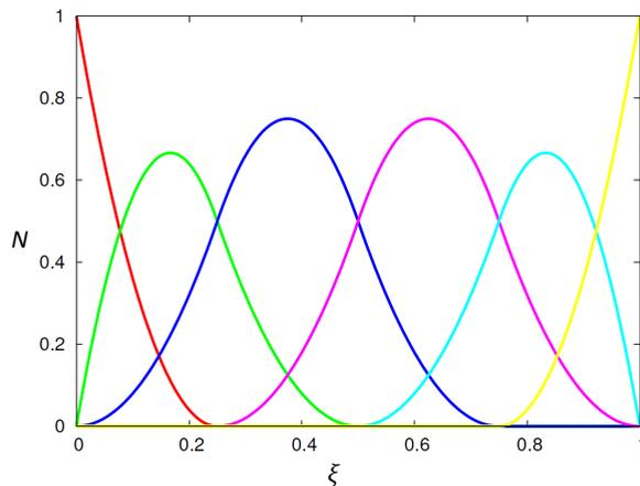
Fig. 1. Quadratic B-spline basis functions for four  $C^1$ -continuous elements with open knot vector,  $\Xi = \{0, 0, 0, \frac{1}{4}, \frac{1}{2}, \frac{3}{4}, 1, 1, 1\}$ .
