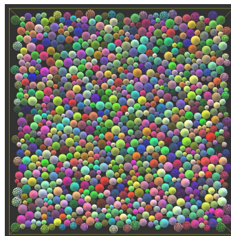
Fig. 4. A sample of the initial configuration of granular packing of a RVE.
