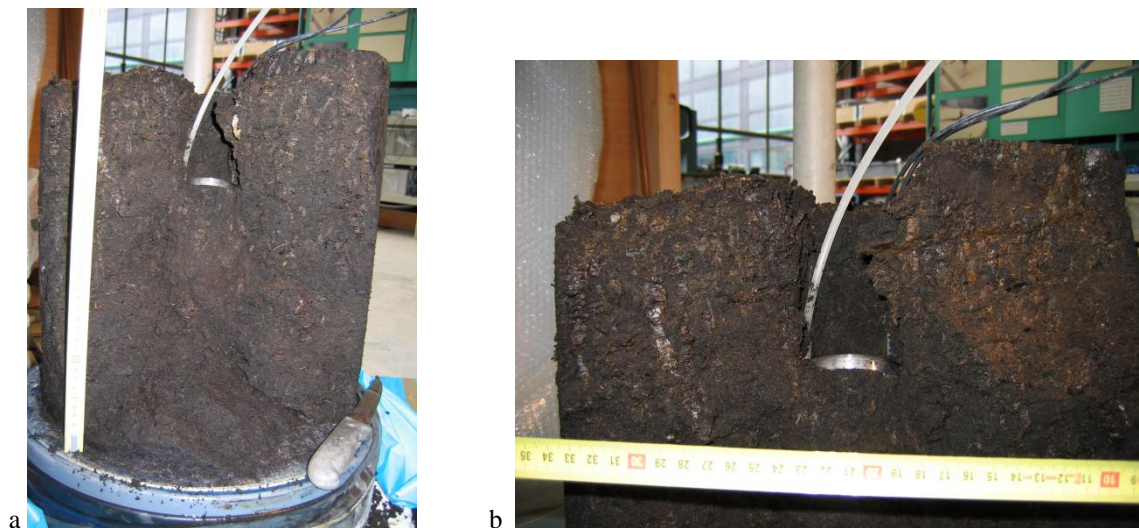
Fig. 9. Impression of plate bearing test results. (a) Peat test 7a. (b) Peat test 7b.
