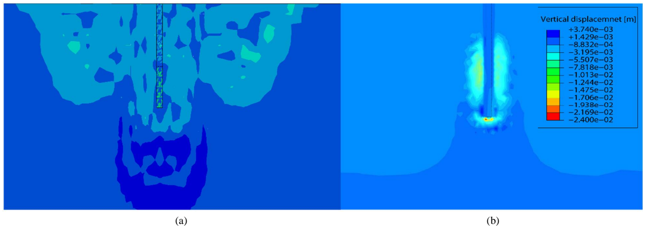
Fig. 8. Vertical displacement of sand after 20 load cycles (a) CEL model (b) MPM model.
